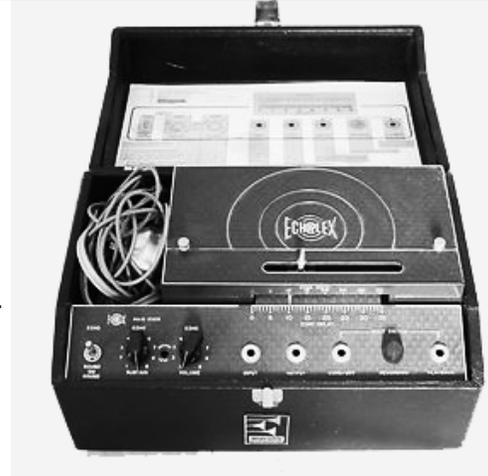
4.) The sound of the tape head traveling across the tape as the Echo Delay slider was manipulated. If you have a lot of repeats going and move the Echo delay slider the echo sound “lags” a bit as the tape head settles into the new position. It’s definitely not a linear behavior like you’d hear in the delay time knobs on most pedals. But it added to the Echoplex mojo and was part of its distinct sound.
